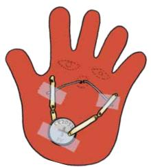
**7. Decorate:** Once the girls' circuit is working, tape the LED and any loose parts to the cardstock/foam, and decorate using markers, pipe cleaners, and other objects.<sup>4</sup>
