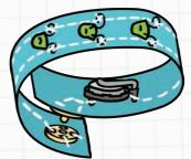
POINTER: If girls have problems, suggest they check all their connections. Then, have them test if the battery and individual LEDs are working. They should also check that the battery is properly inserted into the holder and the LED ends are oriented correctly. Girls may have to cut some stitches and redo a section, but in technology, that's just fixing a bug! Don't let girls get discouraged. 5
